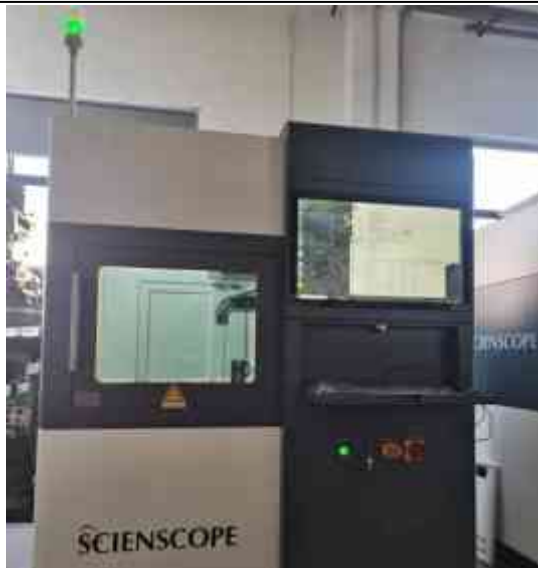
(c) View X2100型自屏蔽式X射线探伤装置
